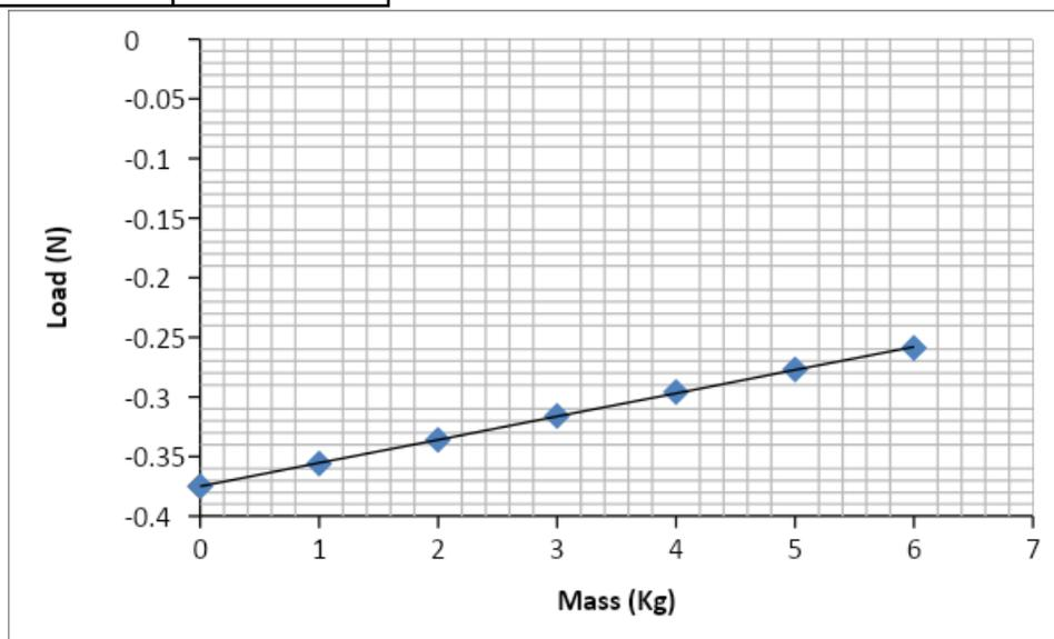
The constant  $K$  is the stiffness and rigidity of the spring. When the force constant is high, the restoring force is also high, and the constant  $K$  is evaluated in  $N/M$ . The  $K$  constant follows Young's modulus compression of springs.
