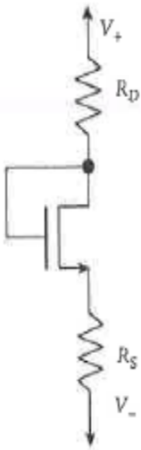
Figure 2: Circuit with a diode-connected NMOS transistor
